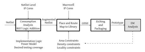
Fig. 1. Description of a typical digital chip design flow. The proposed EM analysis stage is highlighted in gray
