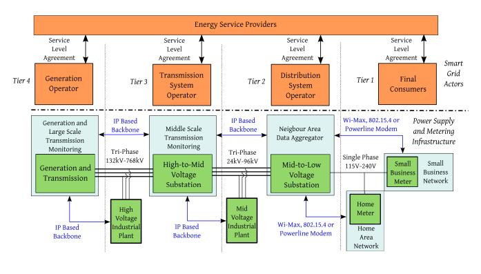
Figure 1. Power supply infrastructure and Smart Grid actors
